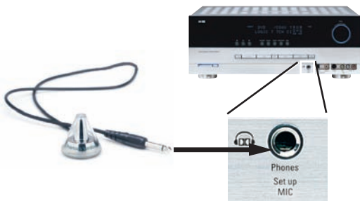
Figure 51 – Plug EzSet/EQ microphone into receiver.
